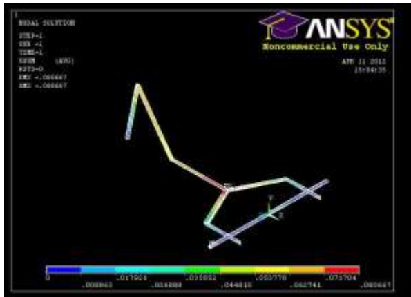
Figure.12 Deflection on Applying Maximum Loads The maximum deflection obtained on application of maximum loads is 0.08066 mm
